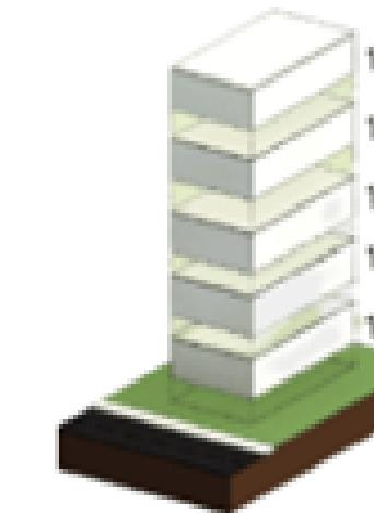
$$CA = \frac{\text{ÁREA TOTAL CONSTRUÍDA}}{\text{ÁREA DO TERRENO}}$$
